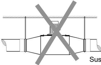
Suspend using the duct part of the housing only!
