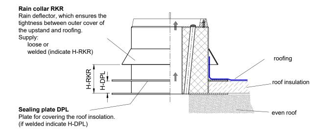
Installation on foundations (upstand preferably with rain water edge)
