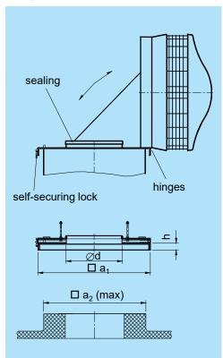
The hinged roof upstand is used if fast access to the ventilation duct or to the fan is necessary, such as for maintenance or duct cleaning. Two profiled plastic plates are connected by hinges and tensioned by self-securing locks. A protective device keeps the open fan safely in position. A profiled seal ensures tight connection to the duct and prevents from soaking of rain water.
