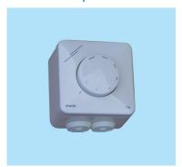
The electronic speed controllers of types ES are used for manual speed control of fans with external rotor motor. Their functional mode is the principle of phase angle control. The integrated switch permits the fans to be turned on and off.
