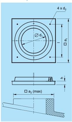
The foundation plate FPL is used for the installation on square foundations, such as brick footing stalls, chimneys, and ducts. It consists of a baseplate with rain collar on which a foundation ring has tightly been screwed and sealed.
