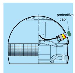
The repair switch RS is used to disconnect the fan completely from the mains in cases of repair and maintenance. This excludes the risk of accidents arising from unauthorized activation.
