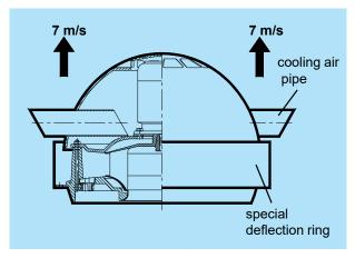
The special version LAB leads to the outlet speed of 7 m/sec. if the following condition is met:
