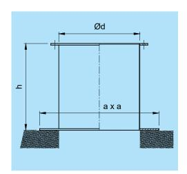
The roof upstand is used for elevated installation of roof fans, such as for compensation of snow heights or insulations.
