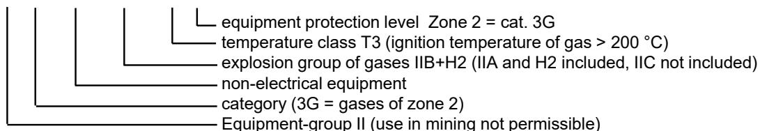
Use in Zone 0 is not possible as a matter of principle. Gases of explosion group IIC (except hydrogen), gases with an ignition temperature below 200°C as well as flammable dusts are also excluded.
