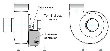
The fans of the VRE...-EC-DR series were developed on the basis of the proven VRE series as a supplement to the variable-speed drives predominantly used for plastic radial fans in the combination of asynchronous motor and frequency converter (version with pressure control). All specifications and notes in the operating instructions "Radial fans VRE" also apply to the use and operation.
