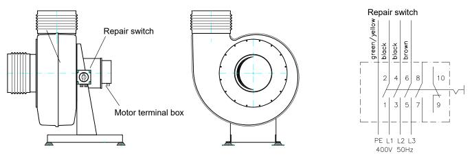
The power supply is connected to the repair switch mounted on the fan.
